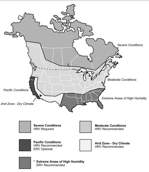
NOTE ERV not recommended where temperatures fall below 25°F (-4°C) continuously for more than 5 days. \*ERV not recommended in regions where high outdoor humidity causes air conditioning operation for dehumidification more frequently than heating system operation.
